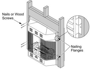
Figure 8 - Attaching Fireplace to Wall Studs
